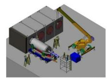
Figure 3.3 Hydraulic Ram Being Aligned to Push a Canister in a NUHOMS Module
