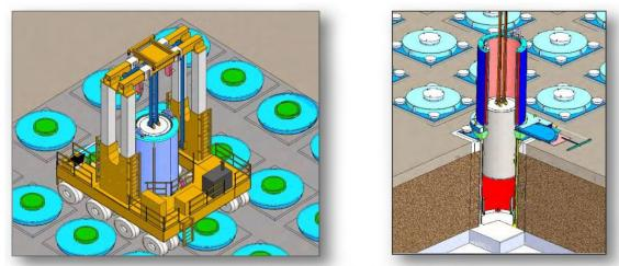
HI-STORM UMAX MPC-37 being Installed in the Underground Cavity
