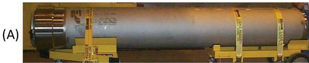
Figure 4-4. Multi-canister overpack and process operations at Hanford.
